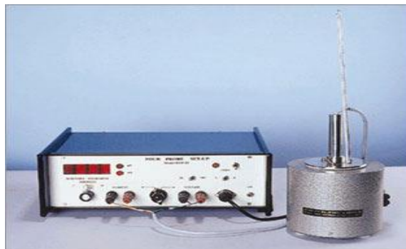
Figure (3): The Four Probes Experimental Set-up
